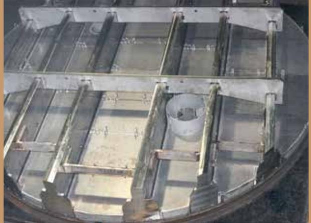
Large Catalyst Support Grid (4000 mm dia.) with Beams and Anti-Buckling Combs
