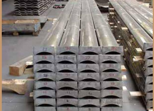
Set of Scallop with perforated liners in AISI 321
