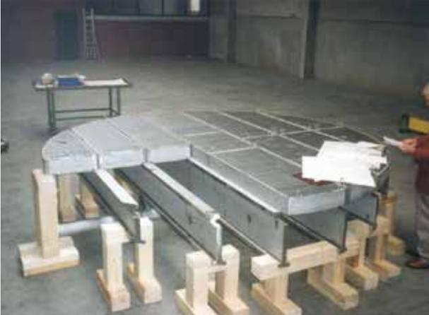
Catalyst Support Grid with Support Beams
