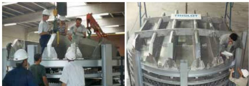
Mock-up Test Assembly of Catalyst Support Grid, Support Beams and HD Tray
